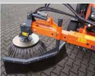
Telescopic, with hydr. inclination adjustment
