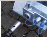
Hitch system and double-acting hydraulic connector (standard)
