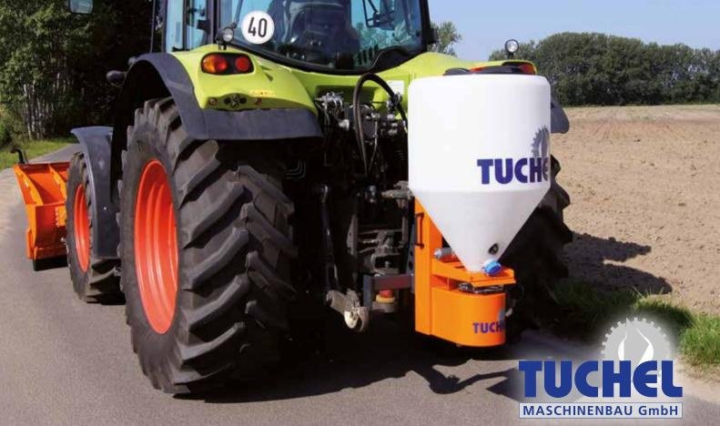
The two salt spreaders **TS 120** and **200** have reservoirs with a capacity of 120 or 200 litres and can be attached in a few simple steps. Driven by a strong geared motor, the spreader can dispense up to 6 m (depending on the material). The speed of the disperser can be adjusted comfortably and easily in the driver's cab.
