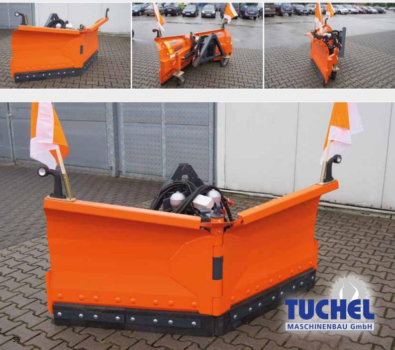
The VARIO snow plow is the ideal machine for a flexible clearing of snow. Hydraulic angling, secured by nitrogen bubbles, allows to use the two-part snow plow in V-, Y- and straight position. The PU-coated (polyurethane) spring flap segments provide security and protect the machine against damage. Infinitely height adjustable wheels assure clearing without leaving any marks on road surfaces. Various hitch systems allow a perfect attachment onto your carrier-vehicle.
