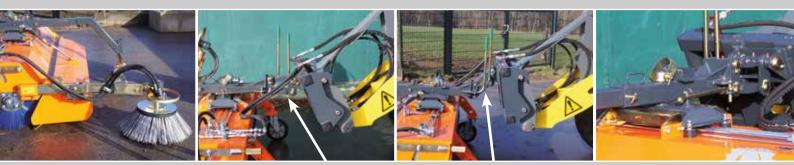
Yard loader / Front loader attachment with parallelogram and pendulum compensation incl. height indicator
